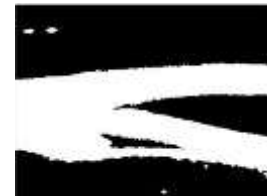
Fig. 8. Segmented binary image obtained by implemented Otsu thresholding algorithm on the pre-processed image.
